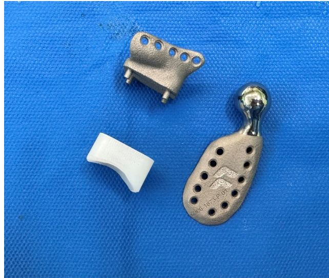
Fig. 2. Ramus-Condyle Unit component was milled from titanium. Fossa component composed of ultra-high molecular weight polyethylene fused to titanium
